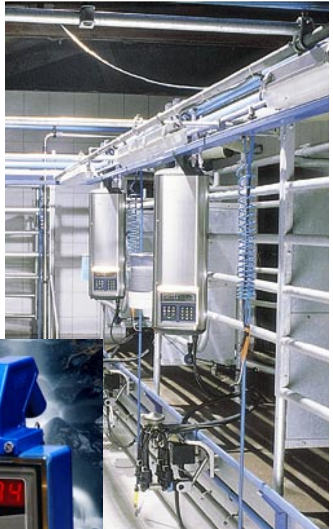
DeLaval milking point MP700 provides you with immediate access to your herd's database.
