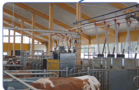
8 automatic feeders in a row in the Feed First barn. Light comes in from the roof ridge ventilation and from the gable.
