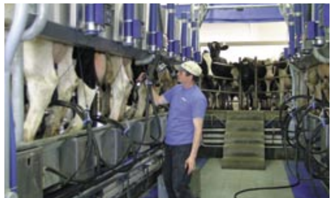
Cascade™ parallel parlour includes necessary features for safe milking, including an air powered index system for correct cow positioning.
