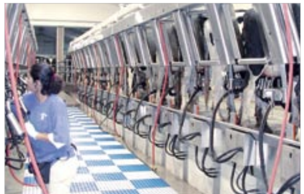
Angled rump rail assemblies improve positioning of each cow while eliminating pressure on sensitive hip pins.
