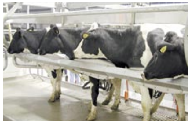
The brisket rail swings up and away from the cows to allow the entire side to exit underneath.
