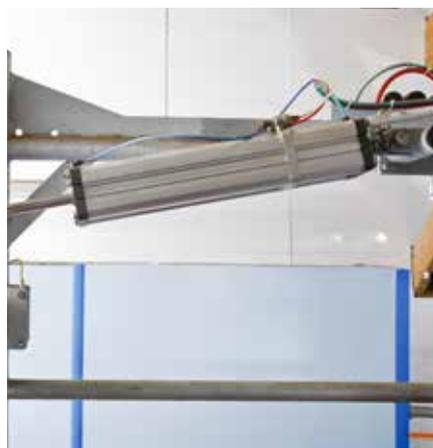
Duplex cylinder for front exit and indexing
