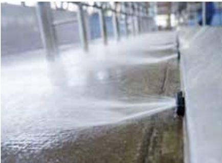
Deck flush nozzles for a clean working place
