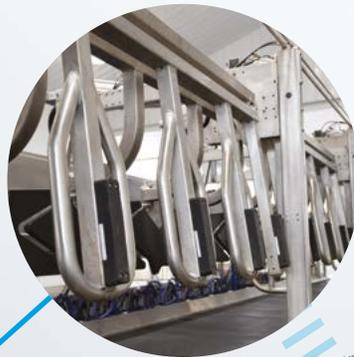
The open bottom design of SynchronoArc™ encourages smooth cow loading.
