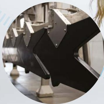
DeLaval SynchroSweep™ delivers a quieter milking process due to the non-overlapping design of the sequence gate.
