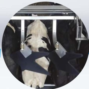
DeLaval SynchronoSweep™ provides an animal friendly method of encouraging cows to leave the milking platform in a timely manner.
